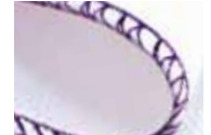
3-thread wrapped overlock narrow Perfect for finishing skirts or as lettuce edge on fine fabrics.
